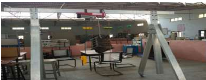
Fig13: Final product, aluminum gantry crane with hoist.
