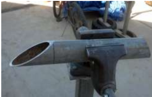
Fig11: Pipe gusset cut.
